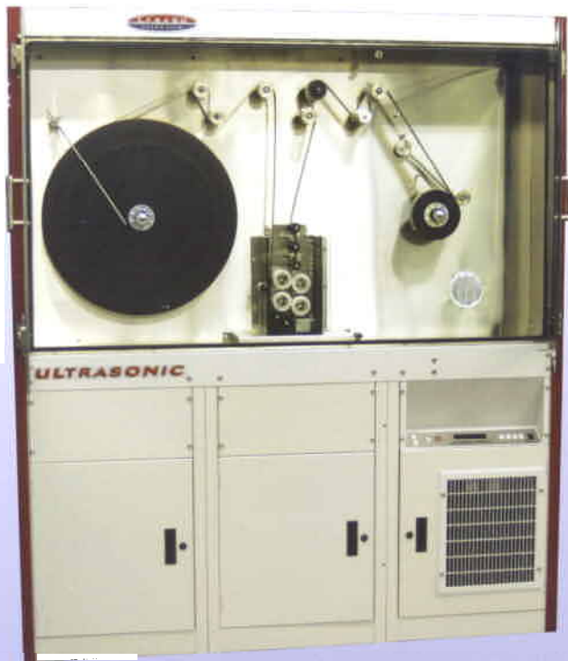
Shown above...the 6000 Foot Capacity Model CF9206 which is also available for use with HFE-8200 or perchloroethylene solvents
